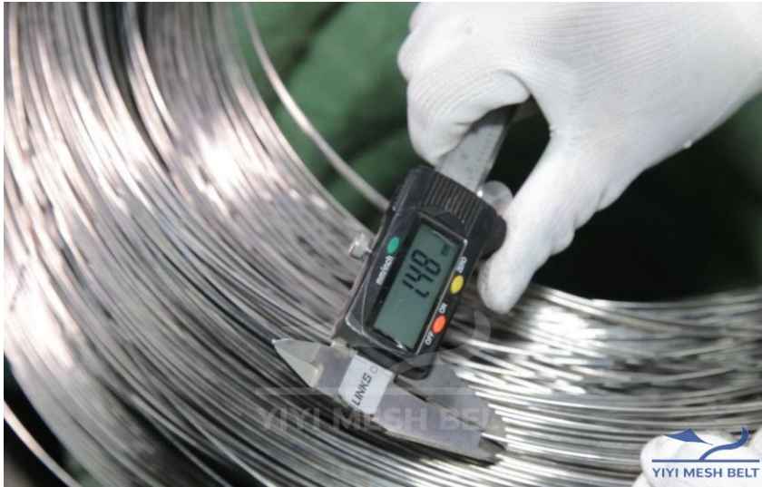
Wire diameter measurement
