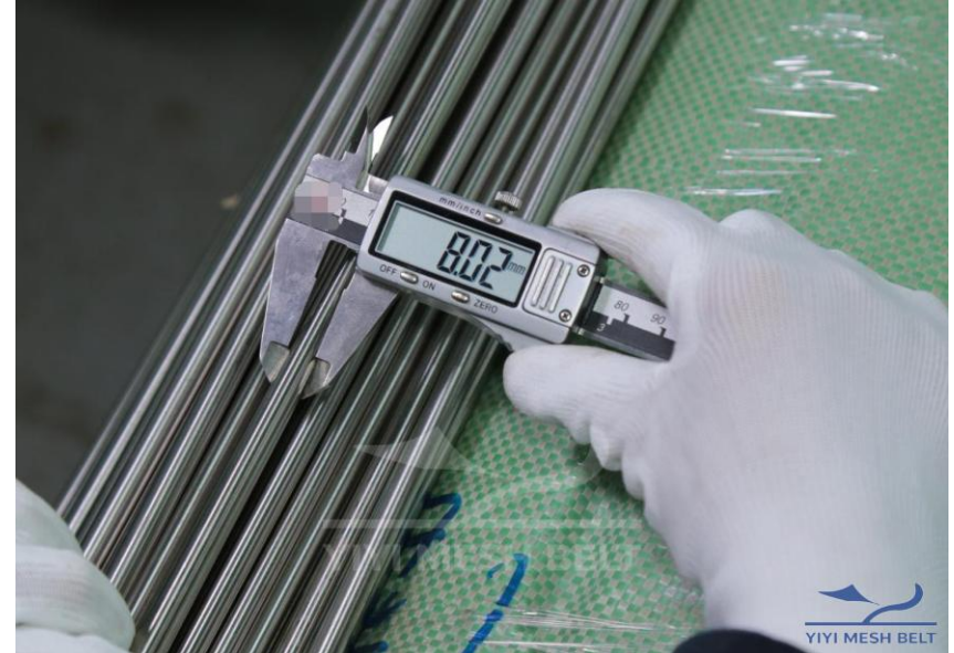
Rod diameter measurement
