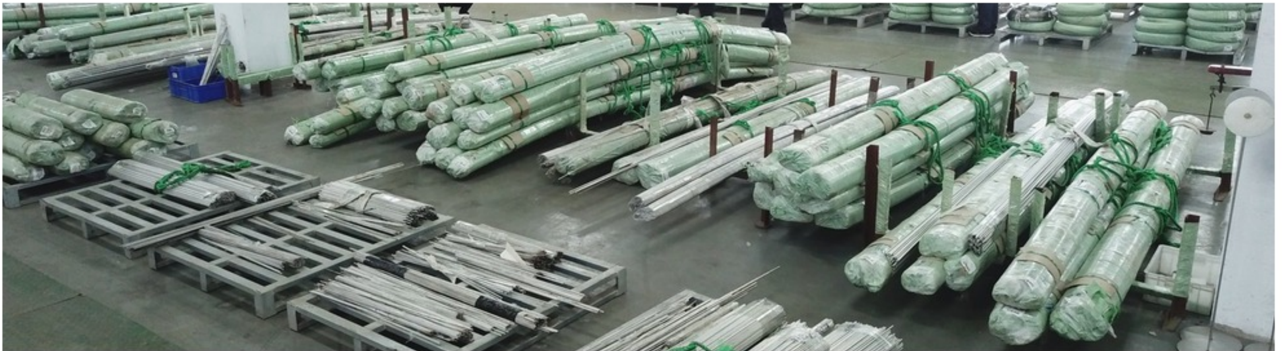
Raw material warehouse: wire rod and bar stored by batch before screening and drawing.
