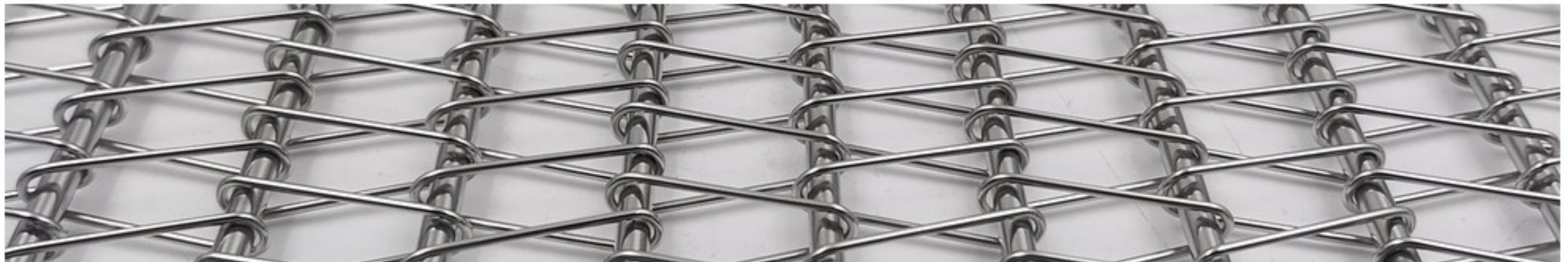
Side links, spiral wire and cross rods: the parts tested in this case.
